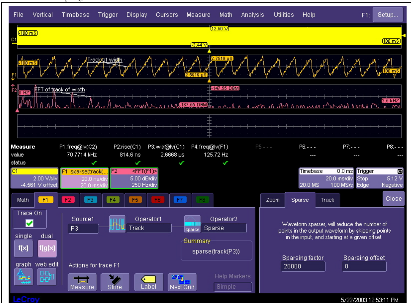
Figure 2 Using the sparsing function to control the FFT span
